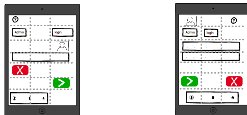
Fig. 3. An illustration of Incorrect layout defect: (left) Incorrect layout ; (right) correct layout.
